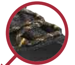
Exposed bridge-lace for gaiter hook
